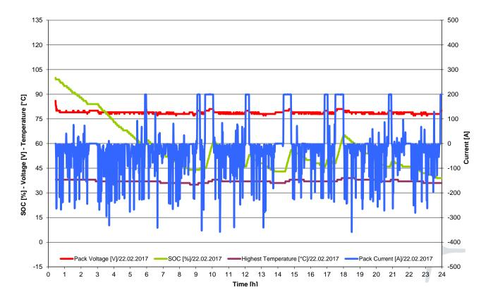
Running a two-shift operation was also tested, and Sonnenschein Lithium handled this scenario comfortably. Under this setup, the forklift was in operation from 6am until 10pm. The battery was charged overnight, and during the day it was charged twice for 30 minutes each. The chart below plots a two-shift operation.
