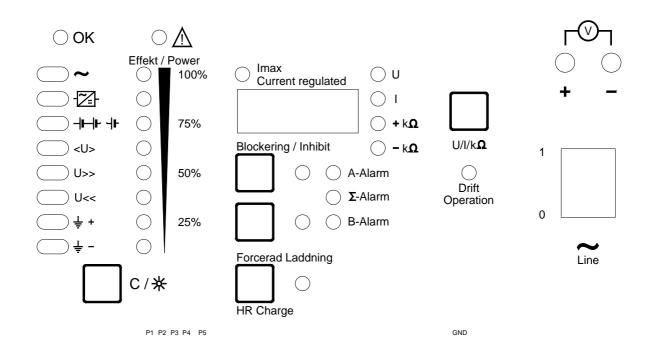
To the right on the front panel there is a **LINE** switch, for controlling power **on - off** of the rectifier. To the left of the switch there is a green LED (Operation) that is on when the power boards are working, and that is normally the same as that there is line voltage present. PLEASE OBSERVE that if the LED is off, this can **NOT** be used as an indication of that there is no voltage present inside the unit.
