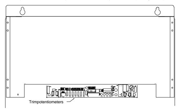
Document 11604/11605 (depending of the units system voltage) shall be available during the adjustment procedure. This is because **only** voltage levels available in this document can be used without having alarms. OBSERVE that if the charging voltage is changed to correspond to a new row in this document, then the alarm board has to be changed accordingly to this new value.
