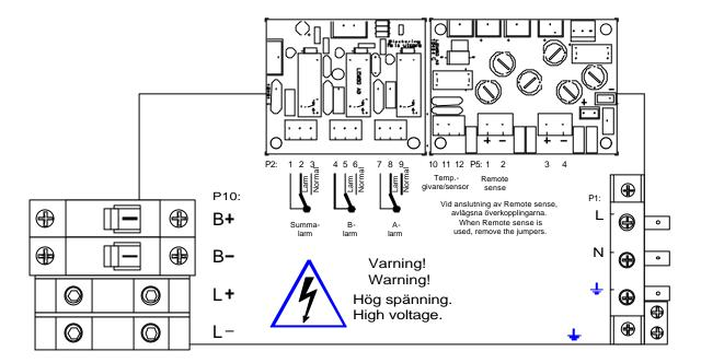
The two automatic fuses that are situated above the battery fuses are the output fuses for the rectifier itself.
