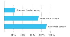
Proven to achieve **90% safe DoD** (compared to 75% for other VRLA batteries). This means more energy available over a longer period of time. Reduced vehicle breakdowns leading to minimized TCO.
