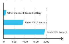
In addition, the Exide GEL range has extremely high parc coverage, more than **2 times** the cycle capacity of the best AGM battery, and even **10 times** more cycles than a comparable standard flood battery.
