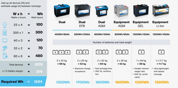
The rated energy in Wh is calculated based on the safe DoD indicated above: 100Ah in AGM is equal to 900Wh because allowed DoD is 75% (otherwise 100Ah at 12V would be 1200Wh)
