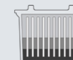
Without Carbon Boost® Sulphuric acid sinks to the bottom of the cell
