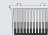
Without Carbon Boost® Sulphuric acid sinks to the bottom of the cell
