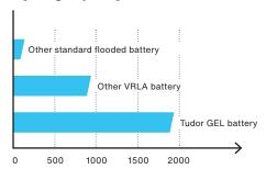
In addition, the Tudor GEL range has extremely high parc coverage, more than **2 times** the cycle capacity of the best AGM battery, and even **10 times** more cycles than a comparable standard flood battery.
