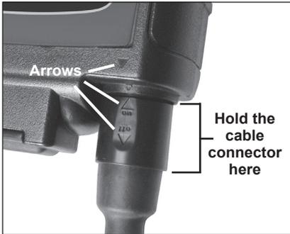
To avoid damaging the battery test cable, always hold the ridged part of the cable connector (as shown in the photo) when inserting and removing the cable.
