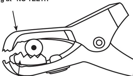
Contact point for testing at “TEETH”
