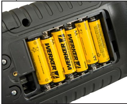
4. Remove the discharged batteries.
