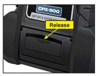
2. Lift the printer door and remove the spent roll.
