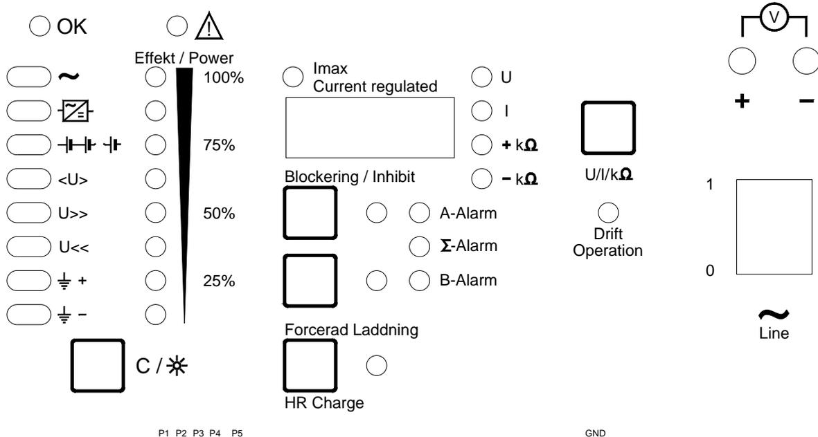
To the right on the front panel there is a **LINE** switch, for controlling power **on - off** of the rectifier. To the left of the switch there is a green LED (Operation) that is on when the power boards are working, and that is normally the same as that there is line voltage present. PLEASE OBSERVE that if the LED is off, this can **NOT** be used as an indication of that there is no voltage present inside the unit.
