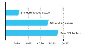
Proven to achieve **90% safe DoD** (compared to 75% for other VRLA batteries). This means more energy available over a longer period of time. Reduced vehicle breakdowns leading to minimized TCO.
