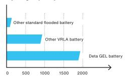
In addition, the Deta GEL range has extremely high parc coverage, more than **2 times** the cycle capacity of the best AGM battery, and even **10 times** more cycles than a comparable standard flood battery.
